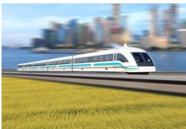
There are even special trains that run on magnets. The tracks become an electromagnet, and they repel the large magnets on the bottom of the train. The train literally levitates over the tracks. The force of gravity is pushed against the opposing magnetic force so the train can float without touching the tracks. This allows it to move faster than a traditional train.
