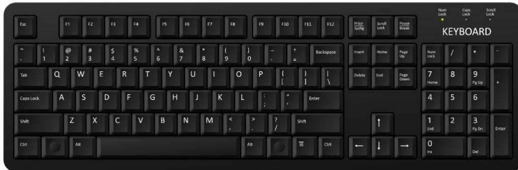
This is a keyboard. It has many buttons on it called keys. We use these keys to type something on the computer. Different keyboards have different numbers of keys, but most standard keyboards have about 105 keys. Different keys perform different tasks.
